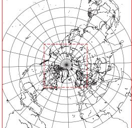
150 km grid size for the hemispheric domain50 km grid size for the Arctic domain
